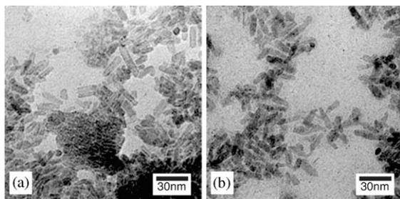
Fig. 1. TEM images of (A) hematite, and (B) maghemite nanorods.
