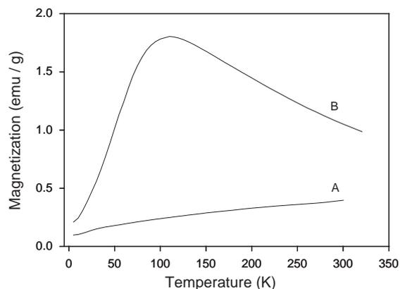
Fig. 3. Magnetization vs. temperature for (A) hematite, and (B) maghemite nanorods with zero-field cooling at the applied field of 100 Oe.
