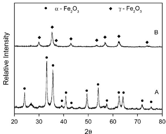
Fig. 2. XRD patterns of (A) hematite, and (B) maghemite nanorods.
