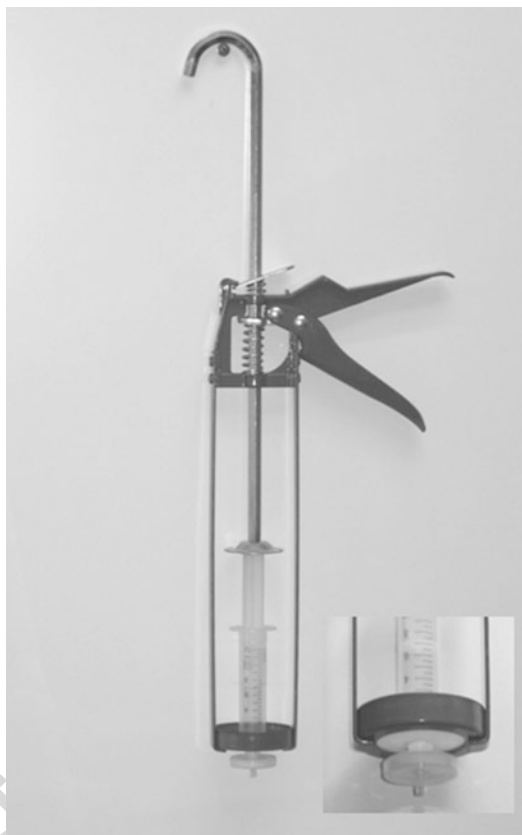
Fig. 6.5 Simple apparatus for filtration of small volumes of polymer solution, based on a sealant gun, a syringe, and a syringe filter with threaded connector
