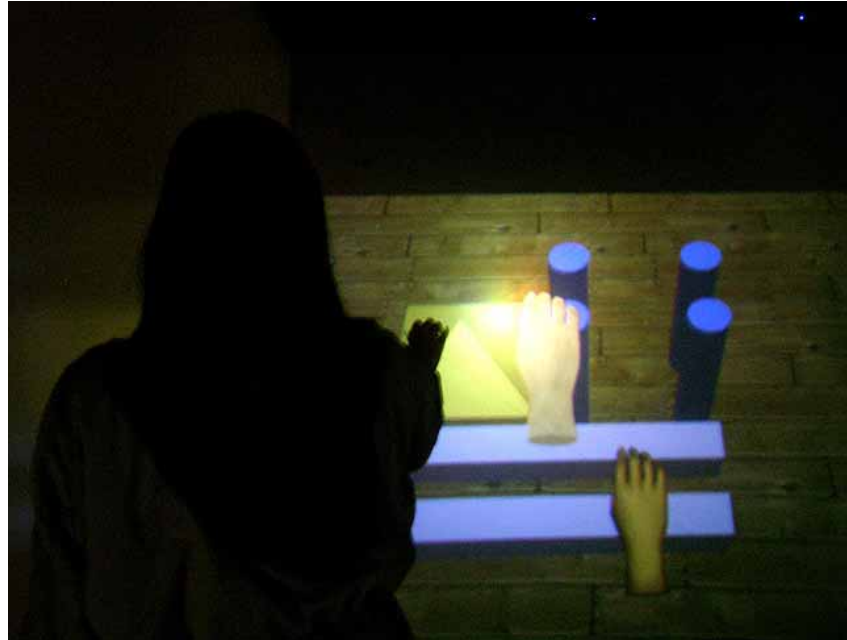
Figure 1. Using the Virtual Dollhouse application, a participant inside the CAVE uses SPIDAR to interact with a PC user.
