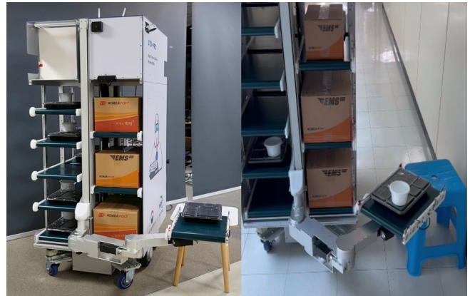
Fig. 1: UTD-pro is a non-contact delivery robot that can deliver lunch boxes and items to isolated residential treatment centers without requiring any physical contact. The robot can deliver twenty items in total on each round. It is equipped with wheels for mobility, a camera for table detection, and an arm for moving items.
